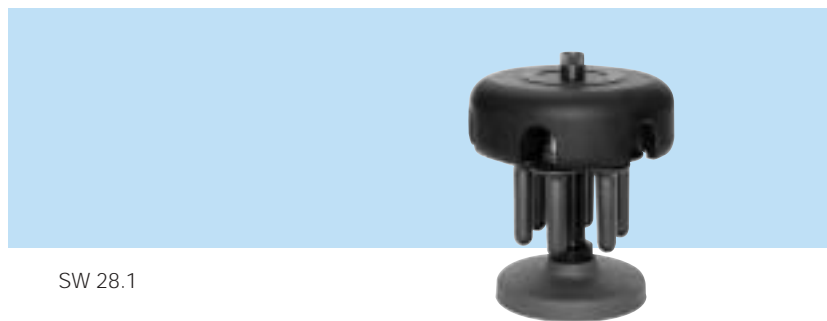
Figure 5-1. Swinging Bucket Rotors
